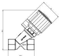
encountered in other piston valves. However, this time, if the flow pressure is too high, the problem of the piston spring does not close the orifice arises. For this reason, the product is not suitable to work at more than 16 bar.
